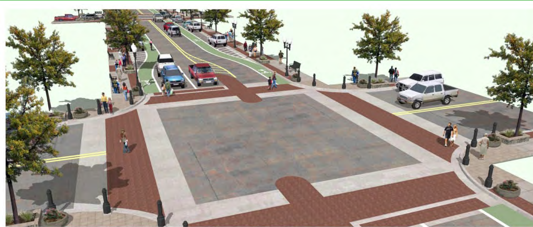
↓ North Avenue Plan View. Right-hand intersection, at 60th and 68th Streets, provides a protected left-turn lane and a surface median refuge for pedestrians. Left-hand intersection is typical, and includes a four-way stop at 64th and 72nd.
