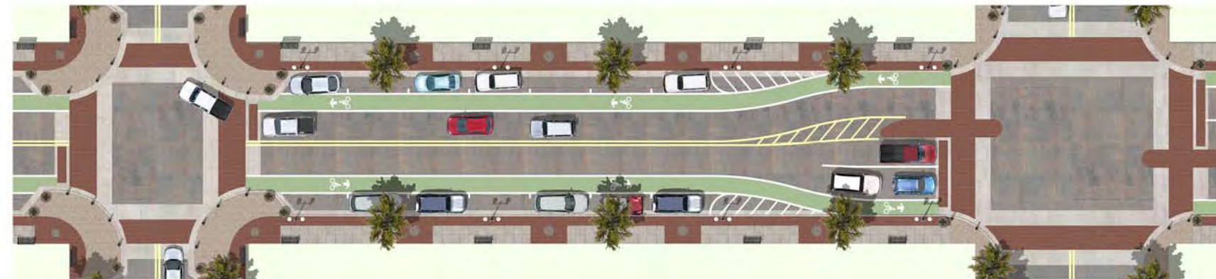
↓ North Avenue Plan View. Right-hand intersection, at 60th and 68th Streets, provides a protected left-turn lane and a surface median refuge for pedestrians. Left-hand intersection is typical, and includes a four-way stop at 64th and 72nd.
